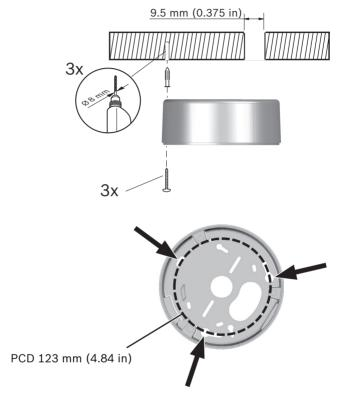
To mount the camera on the surface of a wall or ceiling:
